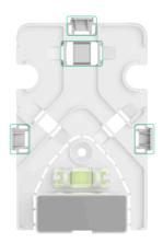
2. Attach the plastic panel to the surface using a bundled screw.
